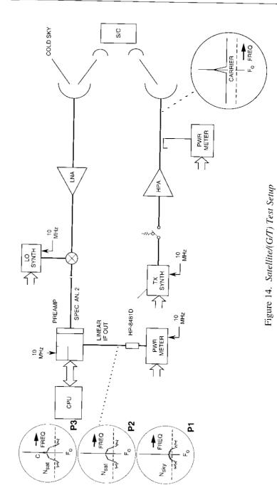
The predicted G/T is calculated based on prelaunch data for the spacecraft receive beam gain and the repeater noise figure, as follows:
