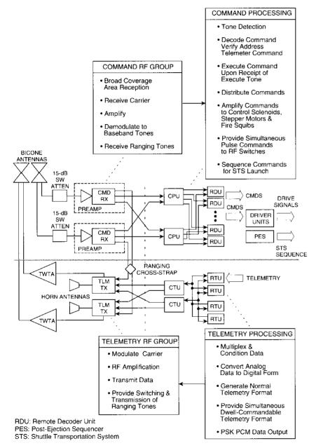
Figure 2. INTELSAT VI Telemetry, Command, and Ranging Functional Schematic
