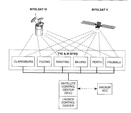
Figure 1. INTELSAT ISCC and TTC&M Sites
