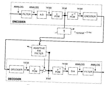
Figure 5. Measurement of Codec Delay
