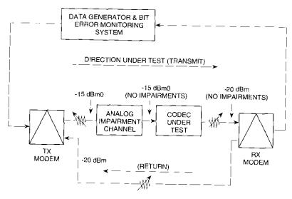
Figure 1. Voiceband Data Modem Test Configuration
