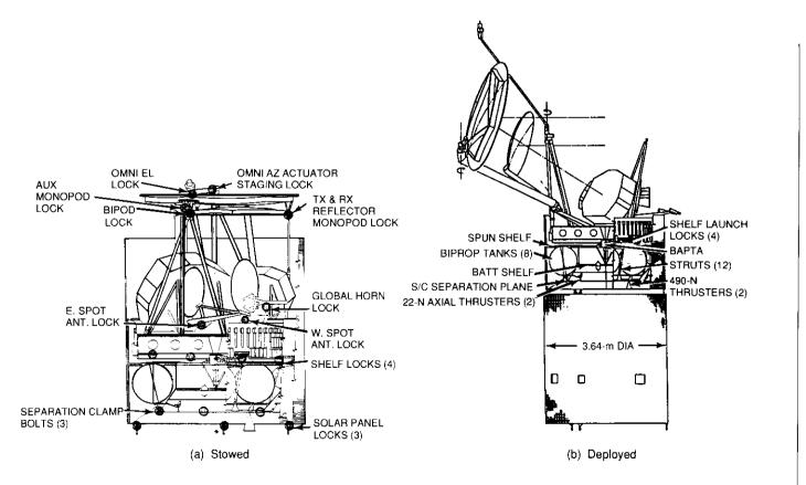
Figure 4. INTELSAT VI Antenna Configurations
