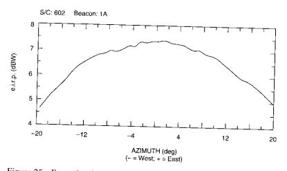
Figure 25. Example of Beacon Co-Polarized Antenna Pattern IOT Result
