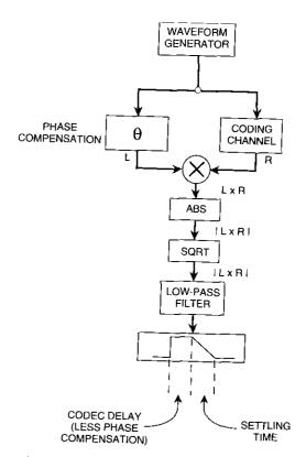
Figure 4. Functional Diagram of V.25 Phase Distortion Measurement Configuration
