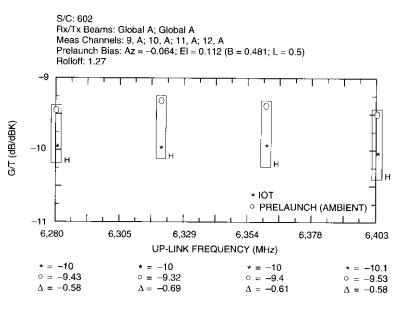
Figure 13. Example of G/T Graphical Test Results
