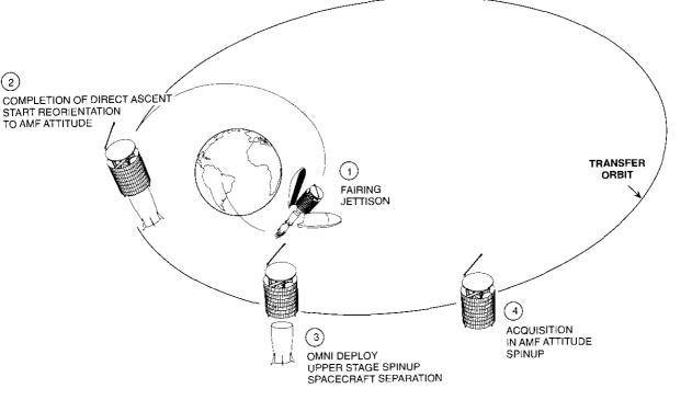
Figure 1. Transfer Orbit Injection
