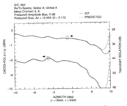
Figure 21. Example of Cross-Polarized Transmit Antenna Pattern Graphical Result
