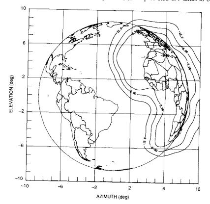
Figure 15. Typical East Hemi Beam-Pointing During IOT Tests
