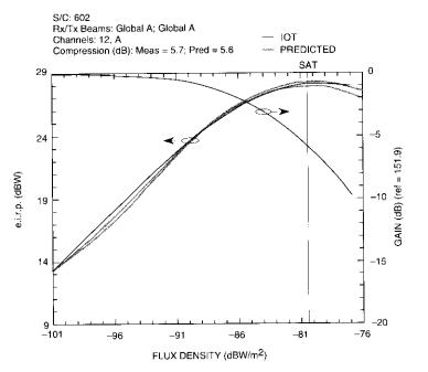
Figure 4. Example of Spacecraft TWTA Gain Transfer Characteristics Data
