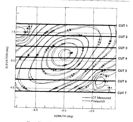
Figure 30. INTELSAT VI West Spot Beam Contours
