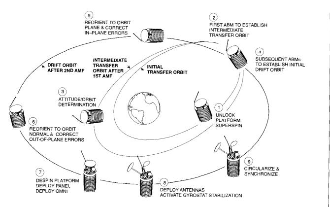
Figure 2. Synchronous Orbit Acquisition
