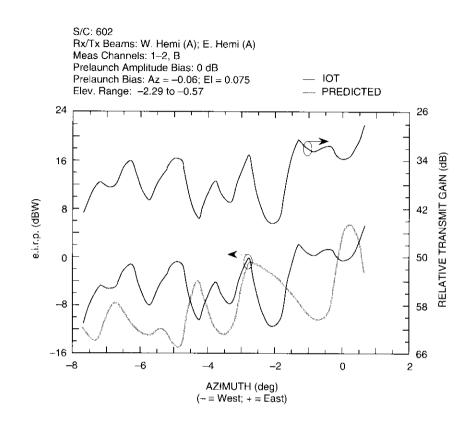
Figure 23. Transmit Sidelobe Graphical Test Result
