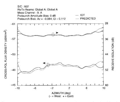
Figure 20. Example of Receive Cross-Polarized Antenna Graphical Result
