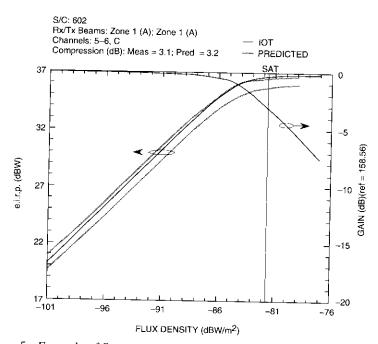
Figure 5. Example of Spacecraft SSPA Gain Transfer Characteristics Data
