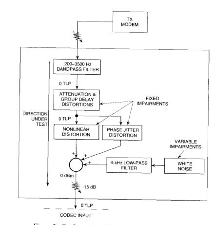
Figure 2. Configuration of the Analog Impairment Channel
