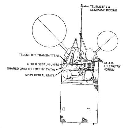
Figure 3. INTELSAT VI Deployed Configuration Showing Location of Some TC&R Subsystem Components
