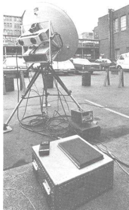
The Labs' transportable antenna, set up in the Cincinnati Chapter's parking lot, enables the Red Cross disaster force to communicate over the CTS satellite with its headquarters in Alexandria through COMSAT's earth terminal in Clarksburg.
