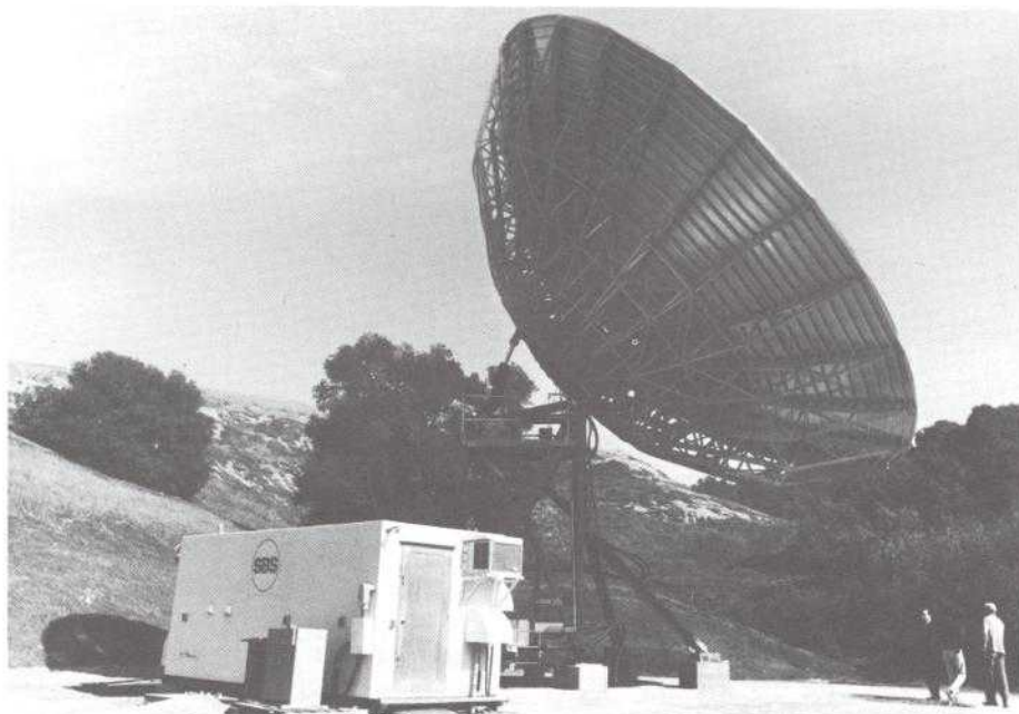
SBS began its preoperational program traffic tests recently using two small earth stations located at Poughkeepsie, New York, and Los Gatos, California, (above photo). The preoperational program is being conducted in the 6 and 4 GHz frequencies, unlike the SBS operational system which will operate in the higher 14 and 12 GHz frequencies.
