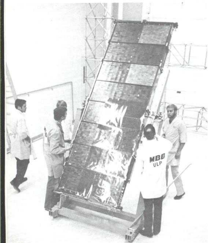
The dolly is designed to tilt the folded solar panels into upright position for hanging on the test track. Light reflections from protective plastic show location of active solar cells.
