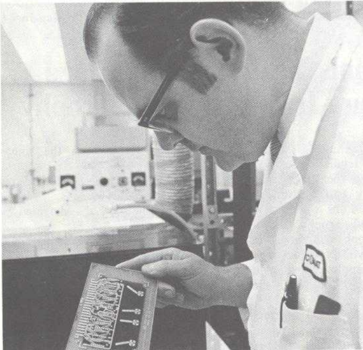
Rocky Lee holds up a rack of boards, just removed from the gold plating tank. The gold on each circuit is worth about a dollar. The addition of gold is the final plating step; it serves to protect the copper beneath from etching and corrosion.
