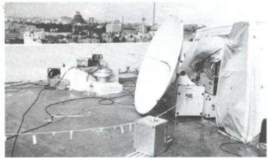
A transportable earth station used by CBS News mounted on the roof of the Intercontinental Hotel in Amman, Jordan.
